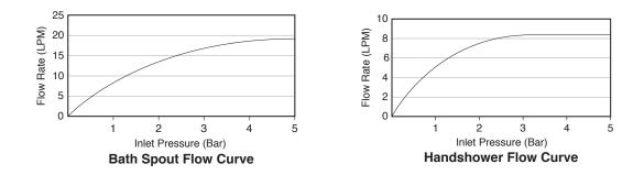
Note: 1. Flow rates are approximate. (1 gallon = 3.785 liters, 1 bar = 14.5 psi) 2. Flow rates shown with supplied flow regulators installed.
