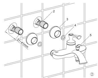
Adjust the center-to-center distance between the connectors to 150mm and horizontally. They should extend 31~41mm beyond the finished wall. Install the escutcheons(3) onto the connectors until they are against the finished wall.
