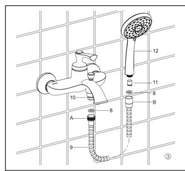
Put the washer(8) into the end A of the hose(9), and connect to the faucet outlet(10).
