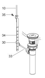
Assemble thumb screw(35) to link(34), and link onto ball lever(33) with 'V'-clip(30).
