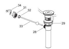
Remove the retaining nut(31) and 'V'-clip(30). Fit the plastic washer (32) and retaining nut onto the ball lever(33). Insert the ball lever assembly into the drain lever hole and through the stopper hole(27). Tighten the retaining nut.
