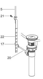
Assemble thumb screw(21) to link(22), and link onto ball lever(20) with 'V'-clip(17).
