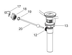
Remove the retaining nut(18) and 'V'-clip(17). Fit the plastic washer(19) and retaining nut onto the ball lever(20). Insert the ball lever assembly into the drain lever hole and through the stopper hole. Tighten the retaining nut.
