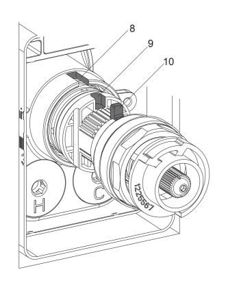
After cleaning, install the cartridge into the body, align the notch(8) of valve body to the notch(9) of cartridge. Make sure the bugle(10) match the notch of the cartridge.
