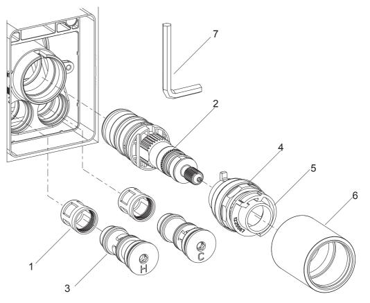
Turn counterclockwise with the hex wrench(7) to uninstall the insert assy(3); Flush and check the filter whether is intact, if damaged replace it; Assemble the filter and insert assy. Tighten the insert and filter kits clockwise with the hex wrench to the valve. **Note:** Make sure that all the parts could not be lost.
