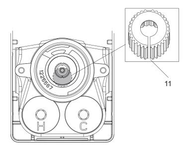
If you turned it without carefulness, you should adjust it and be sure that the notch(11) of adapter is downwards. For accurate temperature, it is supposed to verify and resetting the cartridge according to instruction in previous pages.
