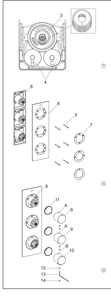
**NOTE:** Don't turn the cartridge spindle during the installation. Ensure that the notch of adapter(3) is downward.
