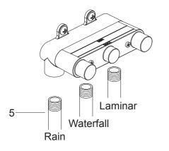
Use appropriate thread sealants or thread tape on the water supplies(5). Connect water supplies to the base.
