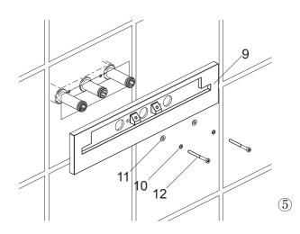
Slide the escutcheon base(9) on the connector till it against the wall, tighten it by screw(12) with washer(11) and locking gasket(10).
