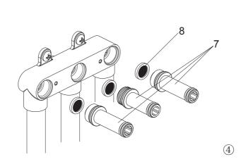
Remove the connectors(7) by hex wrench, take off the filter washers(8). Flush water supplies for about one minute to remove debris. Reinstall the connectors and filter washers.
