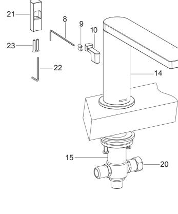
Slide the o-ring(17) into the bottom groove of the escutcheon(16). Tighten the escutcheon with the o-ring onto the diverter kit(15), and keep it against the bath tub. Position the diverter kit so that the nut(20) is on the right. Screw the nut(18). Tighten the screws(19) to secure the diverter kit.
