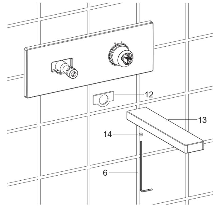
Slide the washer(12) into the groove on the faceplate kit.
