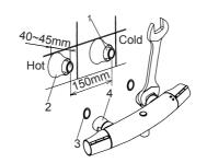
Put the washers(3) into the nuts(4), thread the nuts to connectors. Tighten the nuts with strap wrench or soft cloth between product and regular wrench.
