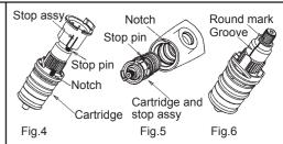
After cleaning, install the "stop assembly" back on the cartridge, adjusting the stop pin into the notch(Fig.4). Install the assembly cartridge and stop in the body, adjusting the stop pin into the notch(Fig.5).
