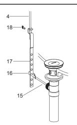
Assemble thumb screw(18) to link(17), and link onto ball lever rod(15) with 'V'-clip(16). Slide lift rod(4) into the hole in link. Push the ball lever down into the open position, and adjust the lift rod. Tighten thumb screw(18).
