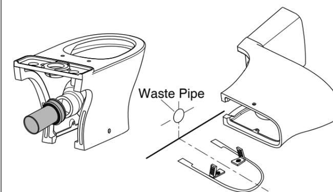
**5** Align connector and carefully lower over brackets.
