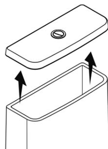
**3** Note the position of the colored buttons for reinstallation.
