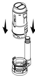
**7** Rotate the canister so that the colored button are in their original positions.
