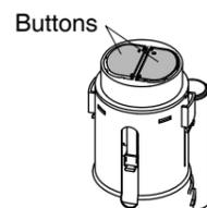
**4** Turn the flush valve tabs and pull straight up on the canister.
