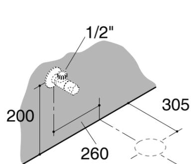
**1** Position the template on the floor to ensure the template against the wall.
