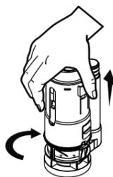
**5** Remove and replace the seal.
