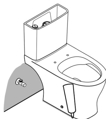
**7** Flush several times and check for leaks. **Do not overtighten!**
