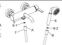
**NOTES:**For 12778T & 72629T, remove the guard on the outlet connector firstly.
