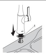
1. Install the gasket(1), foam side down. Install the faucet, the handle is located on the right side.
