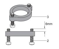
2. Partially thread the screws(2) into the ring(3) until they extend 6mm out the opposite side.
