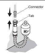
8. Align and connect the spray hose to the connector.
