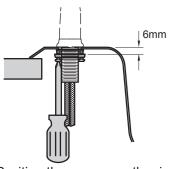
4. Position the screws on the ring onto the shank. Tighten the screws.
