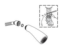
2. To improve the flow, disconnect the sprayhead and clean the screen washer. Reassemble.
