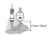
9. Position the weight as shown and tighten securely.
