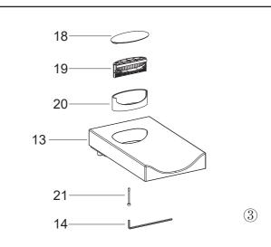
Take out the screw(21) in the bottom of the spout by hex wrench(14). Remove the escutcheon cover(18), rectifier(19) and support ring(20).
