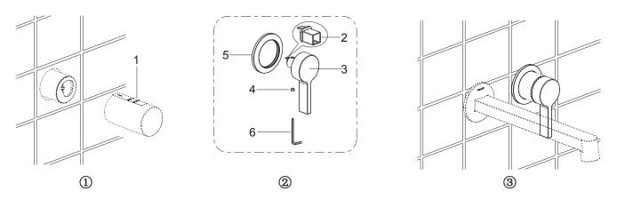
As figure 1 shown, remove and discard the protector(1) after completing the finished wall. Turn off the valve.
