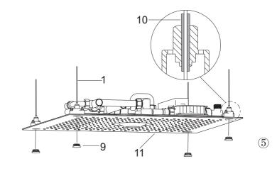
Flush the water supply pipes thoroughly for about one minute to remove debris. Gently pry the caps(9) from the shower head with a tool.
