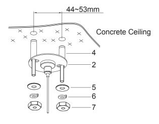
For concrete ceiling, drill eight holes(Ø8mm) at the proper position in the concrete ceiling according to the marked dimensions and expansion screw's(4) diameter.
