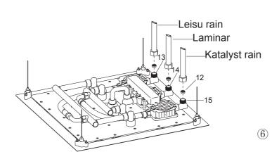
If needed, install the regulator(12) as shown before connecting the hose.
