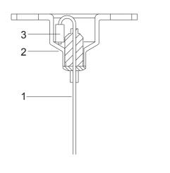
Make sure the end(3) of the stainless steel wire(1) is in the fixing base(2) before installation as shown in the figure.
