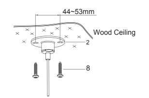
For wood ceiling, install each fixing base(2) along with a stainless steel wire with two screws(8) at the proper position in the ceiling according to the marked dimensions.
