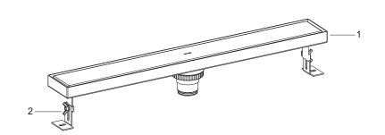
Mount the hidden floor drain(1) according to the determined height. Position it. Adjust the nuts(2) to ensure the drain align with the floor. Fill up the interspace aroud it with cement.
