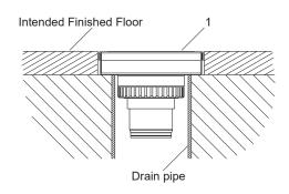
To drain easily, the mounting position of hidden floor drain must be at the lowest area of the whole finished floor.
