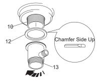
Install the seal(12), secure and tighten the drain body(13) to the waste by hand.
