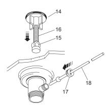
Adjust the drain body to enable the ball lever(18) and lift rod(5) to engage.
