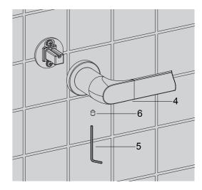
Slide the main body(4) onto the bracket. Orient the screw hole downward. Tighten the screw(6) with the hex wrench(5).
