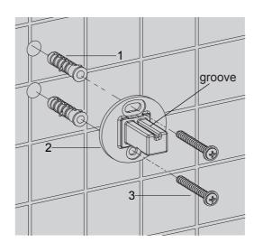
Press the anchor(1) into the hole. Orienting the groove of the bracket upward. Secure the bracket(2) with the self-tapping screw(3).
