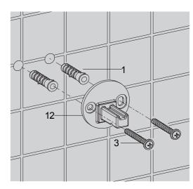
Press the anchor(1) into the hole. Orienting the groove of the bracket upward. Secure the bracket(2)(12) with the self-tapping screw(3).
