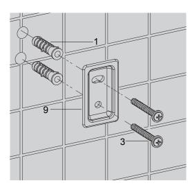
Press the anchor(1) into the hole. Orienting the large slotted mounting hole of the bracket upward, the smaller hole of the bracket downward and two screw holes are vertical. Secure the bracket(9) with the self-tapping screw(3).
