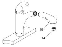
Remove the aerator(14) and the spray(15). Run hot and cold water about one minute to remove any debris. Remove any debris from the aerator and the filter washer of the spray. Shut off the faucet. Reinstall the aerator and the spray.
