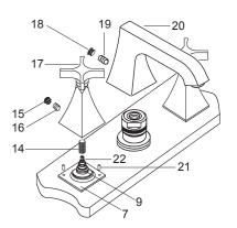
The following configuration shown is the correct position for the installed spout and handles when closed.
