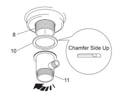
Adjust the drain body to enable the ball lever (12) and lift rod(5) to engage.
