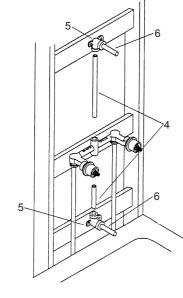
Install G1/2" pipes(4) and ells(5) to the bath and shower outlets. Secure the bath and shower pipes to the support.
