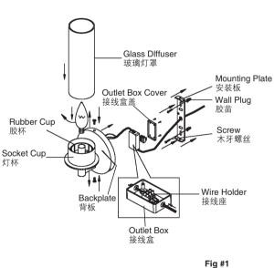
Mark "L" means hot wires. Mark "N" means neutral wires. Mark "≟" means ground wires.
