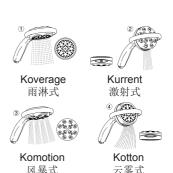
Rotate the head of the handspray to change the spray patterns as shown.
