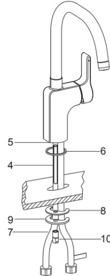
From underside of the sink, place the washer(8), washer(9) and the nut(10) . Position the faucet so that the handle is on the right side. Tighten the nut to secure the faucet to the sink.
