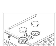
1. When the distance between top surface of bases(2) and bottom surface of tiles is  $\geq$  19mm (bottom surface of tiles is above the MIN line on the protector), and the distance between top surface of base and that of tile is  $\leq$  34mm (top surface of tiles is under the MAX line on the protector):
