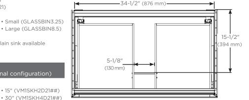
Top view for plumbing and sink clearance
