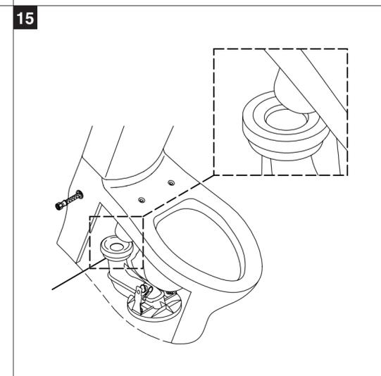
17A. Align the bracket slots with the holes.
