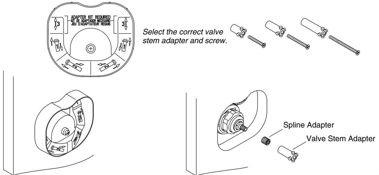
Select the correct valve stem adapter and screw.
